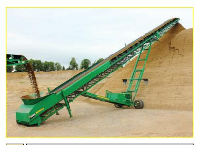
Power Unit: Diesel 49 hp (36.5Kw) Belt: 36" x 80' (915mm x 24.4 m) Stockpile Height: 31' (9.46m) Transport Height: 13'-6" (4m) Transport Length: 57'-3" (17.5m) Stockpile Capacity: 3224 yd<sup>3</sup> (2465m<sup>3</sup>)
